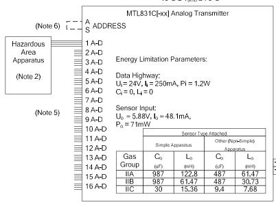
Wire Requirements: Data Highway Plug Terminals: 0.2 - 2.5 mm<sup>2</sup> (12 - 24 AWG) Input Channel and Address Terminals: 0.14 - 1.5 mm<sup>2</sup> (16 - 26 AWG)
