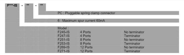
Terminator is a dynamic load for the fieldbus only necessary for the apparatus located at the extremity of the bus.
